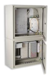
The SI3000 ODU-XS is a small cabinet for FTTB or FTTN deployment scenarios. Compared to other FTTB solutions that require UTP cabling and several Ethernet switches, the SI3000 ODU-XS covers a multi-apartment building from a single location and requires only existing in-house copper cabling. Low investment costs and simple maintenance result in the overall lower operator's TCO.
